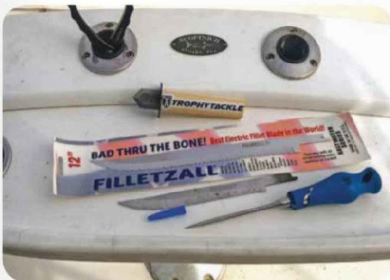
Specialized tools: The Cuda Ice pick is stainless steel, heavy duty and longer than standard pick. The triangular pointed blood drop knife has a guide to ensure perfect depth.
